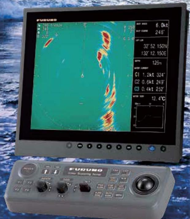
Photo: Control unit with optional monitor MU-150HD
